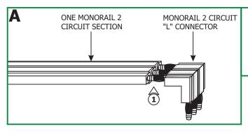
1: Push the Monorail 2 Circuit ceiling "L" connector pins completely into one Monorail 2 Circuit section. Make sure this Monorail section is secured with the standoffs (Refer to the instructions provided with the standoffs).
