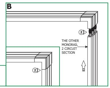
2: Push the other Monorail section completely onto the Monorail 2 Circuit ceiling "L" connector pins and simultaneously connect the Monorail 2 Circuit to the standoffs.
