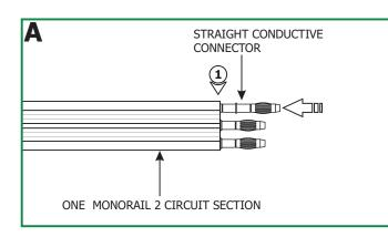
1: Push the Monorail 2 Circuit straight connector pins completely into one Monorail 2 Circuit section. Make sure this Monorail 2 Circuit section is secured with the standoffs (Refer to the instructions provided with the standoffs).
