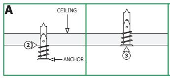
**1:** Hold the Monorail 2 Circuit section against the ceiling or use a plumb bob to mark the standoff locations onto the ceiling (this may require more than one person).
