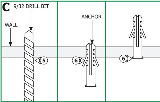
**5:** Use a 9/32 drill bit to make holes on all four marked points.
