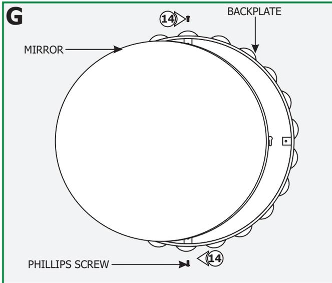
**14:** Align the mirror brackets to the backplate brackets. Place the mirror into the backplate and tighten the Phillips screws to secure the mirror in place.
