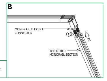
**2:** Push the other Monorail section completely onto the Monorail flexible connector pins and simultaneously connect this Monorail to the standoffs.
