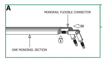
1: Push each Monorail flexible connector pin completely into one Monorail section hole. Make sure this Monorail section is secured with the standoffs (Refer to the instructions provided with the standoffs).
