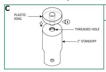
1: (OPTIONAL): If the 1" standoff has the plastic ring attached, then remove the plastic ring and clean the threaded hole.
