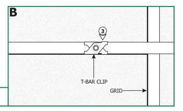
**3:** Place the T-Bar clip onto the grid by squeezing the arms together.
