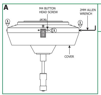
2: While holding the transformer, unhook the transformer cover
