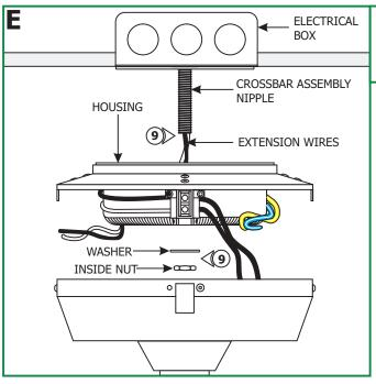
9: Feed the extension wires through the transformer housing center hole. Slide the transformer housing onto the crossbar assembly nipple and secure it in place by tightening the washer and inside nut.
