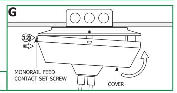
**12:** Hook one of the transformer cover screw holes next to the rectangle cutout, onto the Monorail feed contact set screw.
