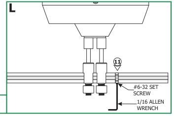
**11:** Tighten the #6-32 set screws on the isolating connectors with the provided 1/16 Allen wrench.
