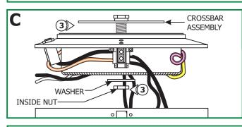
Remove the inside nut and washer to remove the crossbar assembly. DO NOT DISASSEMBLE THE CROSSBAR ASSEMBLY.
