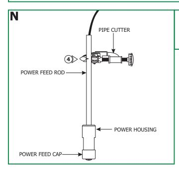
**4:** Use a pipe cutter to cut out the excess rod. If cutting with a hacksaw, then make sure the center wire is removed from the rods. To remove the center wire, remove the power feed cap, pull the wire out. Make sure to clean the burr of the cut section before re-feeding the center wire.
