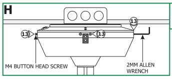
**13:** Place the transformer cover onto the transformer housing. Replace and tighten the five M4 button head screws with the 2mm Allen wrench.
