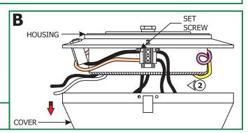
**2:** Unhook the transformer cover from the set screw and remove it from the transformers housing.
