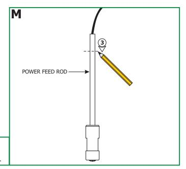
**3:** From the end of the power feed rods mark each rod to the amount that needs to be shorten. For example to resize 24" standoff to 17", mark 7" from the end of the power feed rod.
