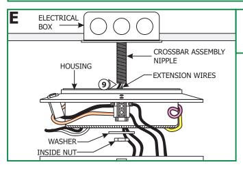
**9:** Feed the extension wires through the transformer housing center hole. Slide the transformer housing onto the crossbar assembly nipple and secure it in place by tightening the washer and inside nut.
