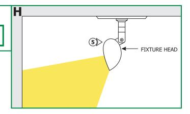
4: Tighten the top M4 set screw with the 2mm Allen wrench to
