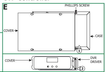
**NOTE:** Use a DVR-RGB-200 (Sold Separately) with this power supply. The power supply and the DVR-RGB-200 are installed on the back of the power supply cover.
