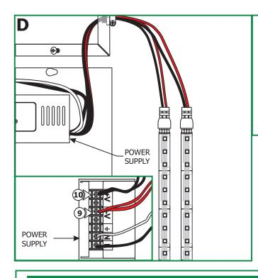
**NOTE:** This power supply is for multiple runs. Do not exceed the maximum wattage of the power supply.
