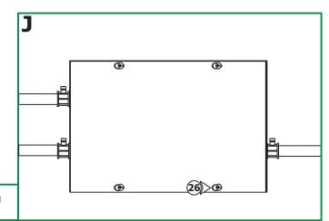
**26:** Replace the power supply cover and secure it by tightening the four Phillips screws.
