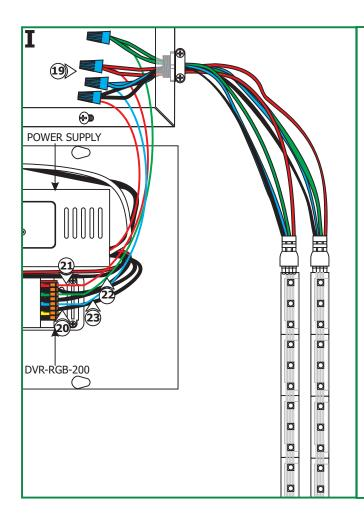
**NOTE:** The DVR-RGB-200 terminals adapt maximum 18 AWG size. To avoid voltage drop, use 6" of 18 AWG size in RGB terminals connected inline to proper size gauge wire attached to the RGB LED wires with wire nuts. See the "Low Voltage Wire Size Chart" on page 1.
