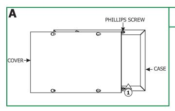
**1:** Loosen the four Phillips screws on the front of the power supply cover to slide the cover off of the case.
