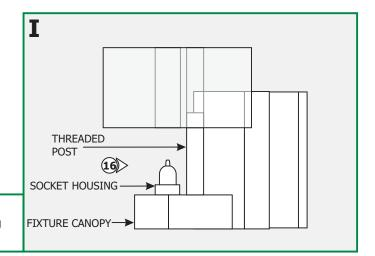
**16:** Slide the glass diffuser back hole onto the threaded post. Align the glass diffuser center hole with the socket housing and carefully rest the diffuser onto the fixture canopy.
