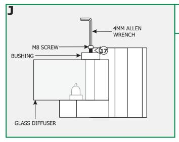
**17:** Replace the bushing and M8 screw onto the threaded post. Tighten the M8 screw with the 4mm Allen wrench to secure the glass diffuser in place.
