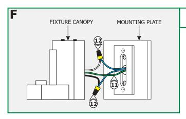
**12:** Connect each transformer low voltage wire (blue wire) to one fixture wire with a wire nut.
