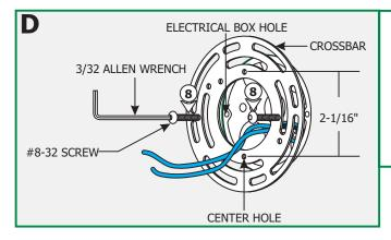
**NOTE:** The two center mounting holes (spaced 2-1/16" apart) on crossbar should be oriented vertically when mounting the crossbar to electrical box.
