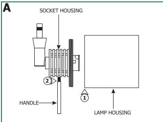
**<u>CAUTION:</u>** To reduce risk of a burn or electrical shock during lamping, disconnect the power to the fixture.
