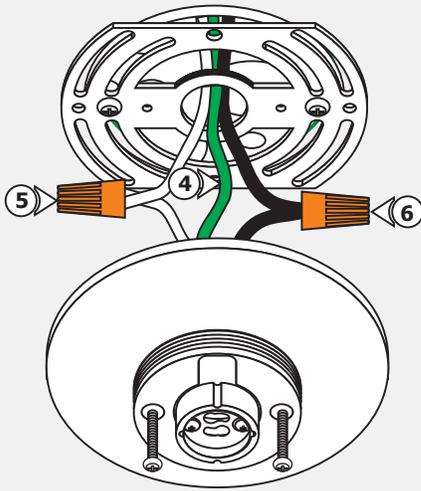
**4:** Make sure the fixture is grounded in accordance with local electrical codes.
