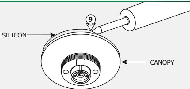
**9:** For installation in **wet location**, caulk around the fixture canopy with waterproof construction sealant.
