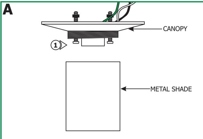
**1:** Loosen and remove the metal shade from the canopy.
