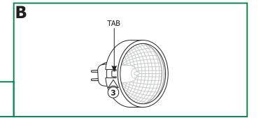
**3:** Press the tabs on sides of the snap lens holder against the MR16 lamp to keep it in the position.
