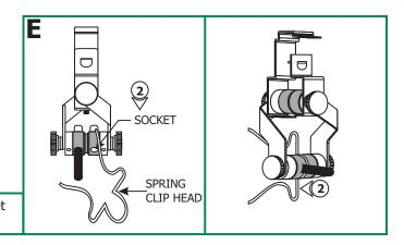
**2:** Push the spring clip completely onto the center of the socket groove until it snaps in place.
