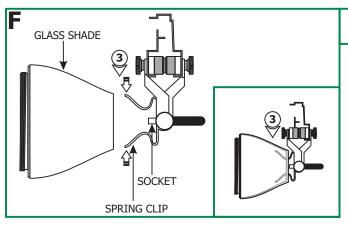
**3:** Squeeze the spring clip ends while inserting it into the glass shade.
