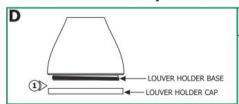
**1:** Unscrew and remove the louver holder cap from the louver holder base.
