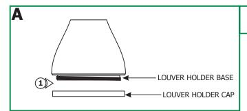
**1:** Unscrew and remove the louver holder cap from the louver holder base.
