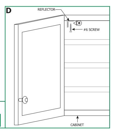
**8:** Place the reflector on surface and secure with the provided #6 screws.
