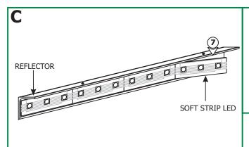
**NOTE:** Avoid bending the soft strip in sharp horizontal angles which may damage the LEDs. Use the proper power connectors.
