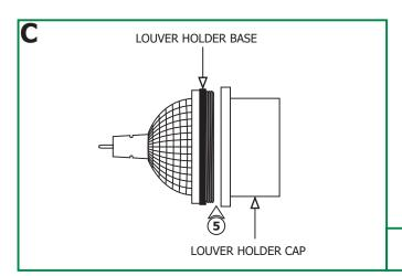
**5:** Tighten the louver holder cap to louver holder base.
