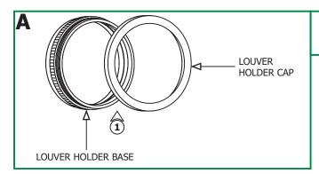
**1:** Unscrew and remove the louver holder cap from the louver holder base.
