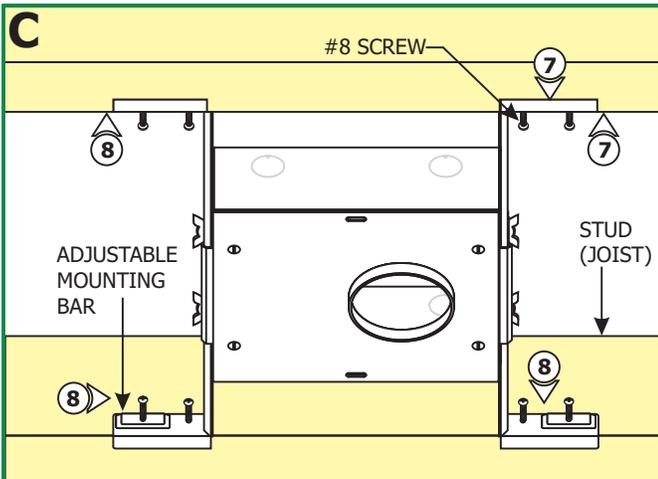
**NOTE:** The adjustable mounting bars mount to joists (studs) that are spaced 16" to 24" apart.
