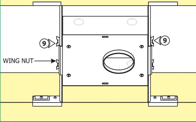
**9:** Slide the housing to desired position. If necessary loosen the wing nuts to ease the sliding. After the desired position is achieved tighten all the wing nuts.
