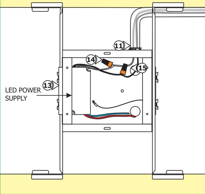
**11:** Remove a knock out to install the power line conduit.
