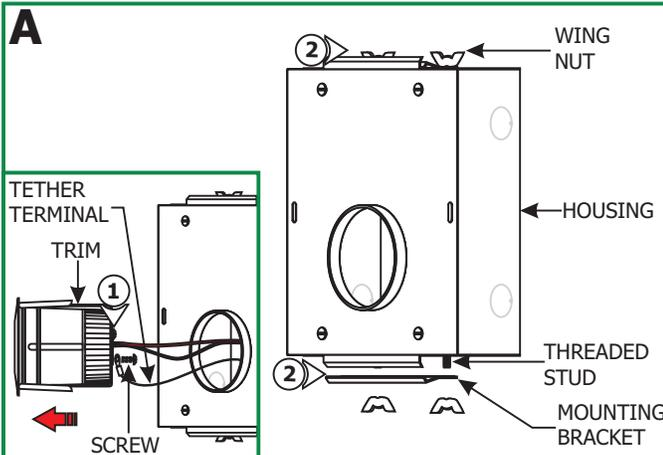
**1:** Carefully pull the trim out of the housing, and remove the Phillips screw on the tether terminal (safety cable) to release the trim.
