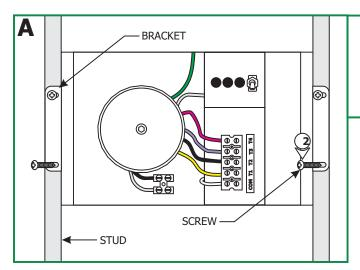
1: Install two THHN low voltage wires from the transformer to the electrical box to which the power feed canopy will be attached. Run the proper size wire using the "Low Voltage Wire Size Chart" below.
