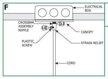
**12:** Slide the canopy into the crossbar assembly nipple and secure using the strain relief.
