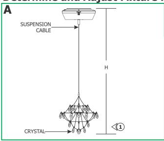
**1:** Push the suspension cable into the center mounting standoff to determine the desired height from the mounting surface of the power supply to the bottom of the fixture. Refer to Figure H for more details.
