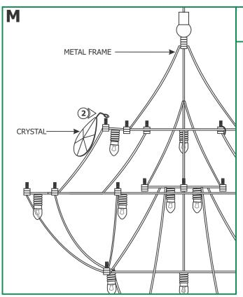
2: Secure each crystal loop to a threaded post on the metal frame. Repeat until all crystals have been mounted to the metal frame.
