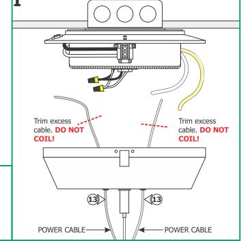
**13:** Feed one fixture power cable through each grommet opening in the power supply canopy.
