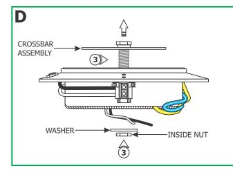
**3:** Remove the inside nut and washer to remove the crossbar assembly. **DO NOT DISASSEMBLE THE CROSSBAR ASSEMBLY.**
