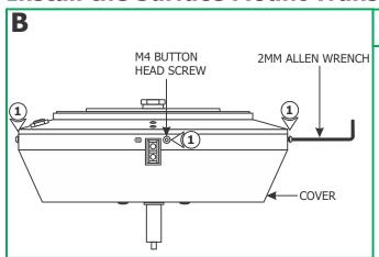
**1:** Loosen and remove the five M4 button head screws around the transformer cover with the provided 2mm Allen wrench.
