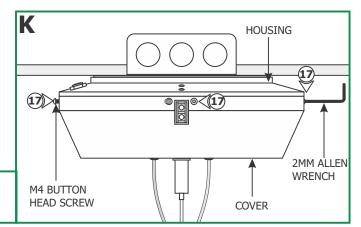
**Install the Lamps and Crystals**
