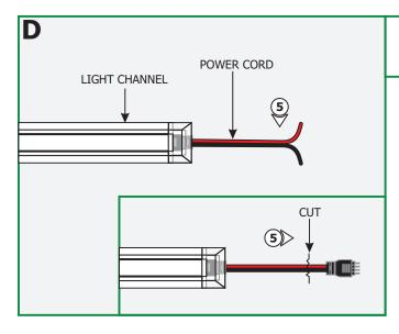
**5:** Cut the other end of the power cord (male or female) and discard it. Strip the wire end for connecting it to the power supply.
