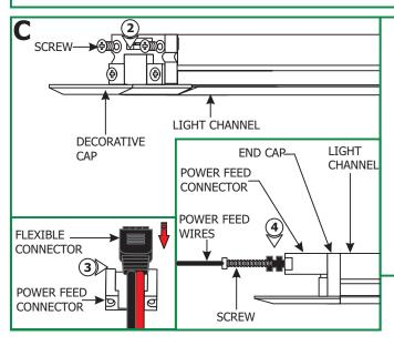
**NOTE:** The power feed cable can be mounted to either the female or male end of the channel.
