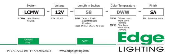
Application: Electronic low-voltage dimming for 2.3W/12V Light Channel Millwork
