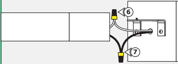
**6:** Connect the white fixture wire to the neutral power wire with a wire nut.
