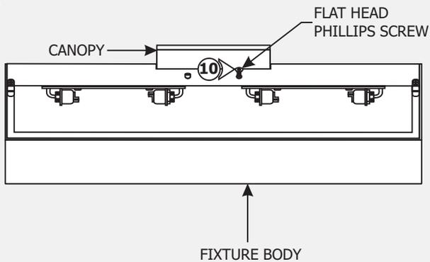
**10:** Secure the other fixture body hole with the flat head Phillips screw provided.
