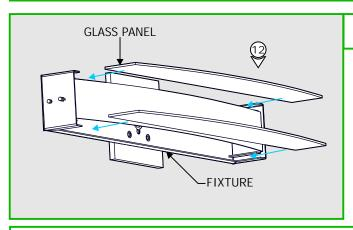
12: Slide the glass panels into top and bottom of slots of the fixture.
