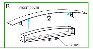
2: Remove the front cover from the fixture.
