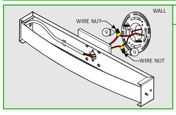
9: Connect each fixture wire to one red LED driver wire using wire nuts.
