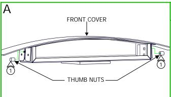
1: Remove the two thumb nuts on the sides of the fixture body to detach front cover.
