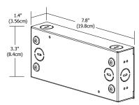
**Description:** LED power supplies transform and regulate power from a line voltage power source into low voltage power for use with LED lighting. The PSB-60W-ELV-24VDC power supply accepts input voltage in range of 120 volts AC and outputs 24 volts DC power up to 60 watts. The power supply can be used as a dimmable or non-dim power supply.
