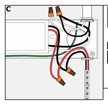
**NOTE:** In order to use small gauge wires from the power supply to the LED fixture, it is recommended to install the power supply as near as possible to the LED fixture. See "Low Voltage Wire Size Chart" below.
