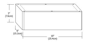
**Description:** LED power supplies transform and regulate power from a line voltage power source into low voltage power for use with LED lighting. The PSB-100W-24VDC-RGB power supply accepts input voltage ranging from 100-277 volts AC and outputs 24 volt DC power up to 100 watts. The integrated RGB Driver receives signals from CDP or CTP to control RGB color mixing and light intensity.
