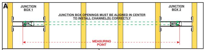
**NOTE:** Select the location between the two studs where the channel is going to be mounted. Each end of the channel must be into an junction box opening. One junction box is used as the power feed and the other one for excess soft strip.
