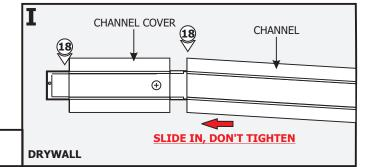
**18:** Insert the channel into the channel cover ends and carefully insert into the drywall slot.
