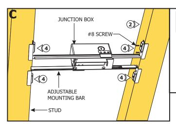
**NOTE:** The adjustable mounting bars mount to studs that are spaced 16" to 24" apart.
