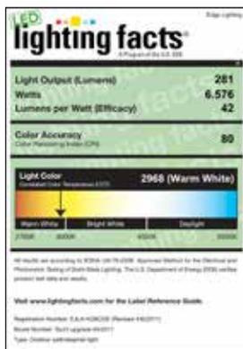
Lighting Facts Label reflects test data for Sun3 with 16 degree lens (L1). See Lamp Specification section above for additional details.
