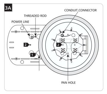
**1** Feed the power line wire through the conduit connector into the pan.
