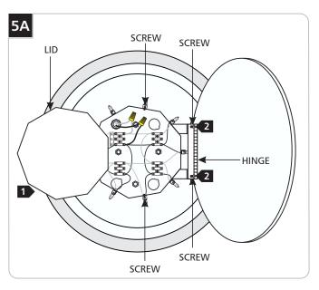
Replace the lid onto the electrical box and tighten the two screws.
