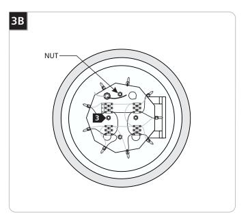
3 Tighten the four provided nuts to secure the pan onto the back plate.
