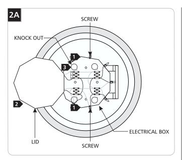
1 Loosen (do not remove) the two screws on side of the electrical box in the center of the pan.
