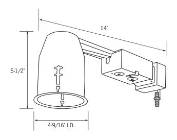
Ceiling Opening: 4-1/8" Max. Ceiling Thickness: 1-1/4"
