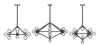
**NOTE:** Determine the desired overall fixture height using the 8" stem only or using additional combination of 20" and 12" stems for a maximum overall extension of 74".
