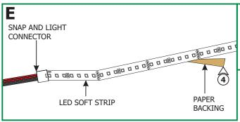
**4:** Carefully remove the backing from the LED soft strip, make sure not to remove the tape from the soft strip. Firmly press down the adhesive portion of the soft strip onto the mounting surface while removing the rest of the backing, making sure there are no air bubbles that can cause surface irregularities.
