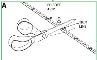
1: If necessary trim the LED strip at the marked line above the contact (every 4" apart) with a sharp scissor to fit the design.
