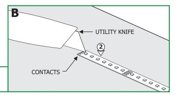
2: Place the LED Soft Strip on a flat, stable surface. Using a utility knife, carefully scrape the protective coating from the contacts.
