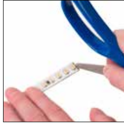
Scrape protective coating from contacts
