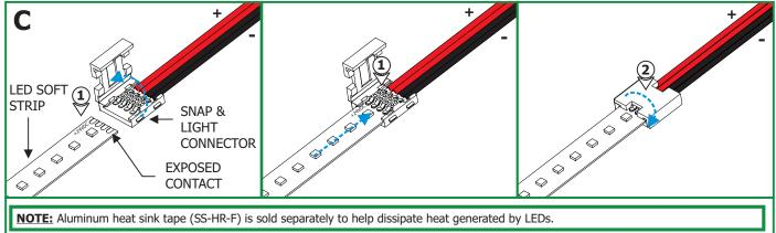
1: Align the +24VDC marking on the soft strip with the red wires of the Snap & Light connector. Insert the exposed contact at the end of the LED strip under the Snap & Light contacts ensuring that the strip contacts are aligned and covered under the connector contacts.
