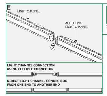
**NOTE:** Multiple light channel can be connected together directly by connecting male end of one to the female end of the other one, or by using the flexible connectors up to a maximum of 25 feet.
