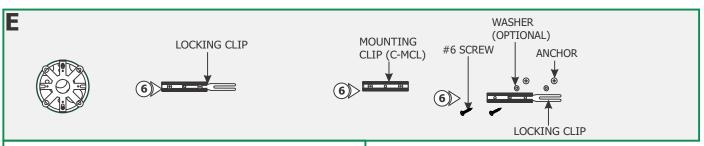
**6:** Line up the locking clips & mounting clips to anchor holes and secure them by tightening the two #6 screws through the clip holes followed by the washers into the anchors.
