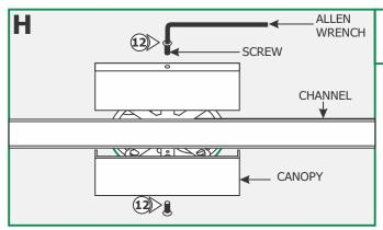
**12:** Place each canopy piece against the channel & line up the canopy hole with the crossbar hole. Secure the canopy in place with the screw & Allen wrench provided.
