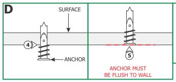
**NOTE:** Steps 3 and 4 are for drywall mounting. Omit these steps if mounting the clips to a wood surface directly.
