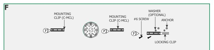
7: Line up the locking clips & mounting clips to anchor holes and secure them by tightening the two #6 screws through the clip holes followed by the washers into the anchors.
