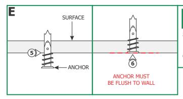
**NOTE:** Steps 5 and 6 are for drywall mounting. Omit these steps if mounting the clips to a wood surface directly.
