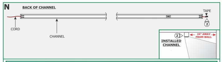
**NOTE:** Remote power supply must be installed within 40ft of Junction box. The low voltage 24V DC wires must be present in Junction box before installing the channel. Refer to the installation instructions provided with the power supply. See page 6 for wiring diagram.
