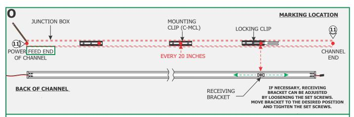
11: Lay the channel to the desired location & make all necessary markings which will consist of the channel ends, locking clips and mounting clips. Mounting clips must be installed every 20" from each locking clip, locking mounting clips are not necessary for channels under 2ft.
