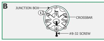
**1:** Mount the crossbar to the Junction box holes with the two #8-32 screws provided.
