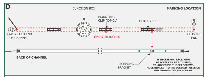
**3:** Lay the channel to the desired location & make all necessary markings which will consist of the channel ends, locking clips and mounting clips. Mounting clips must be installed every 20" from each locking clip, **locking mounting clips are not necessary for channels under 2ft.**
