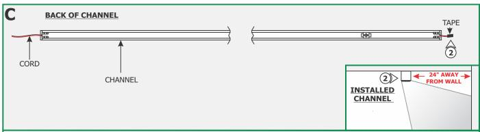
**NOTE:** Remote power supply must be installed within 40ft of Junction box. The low voltage 24V DC wires must be present in Junction box before installing the channel. Refer to the installation instructions provided with the power supply. See page 7 for wiring diagram.
