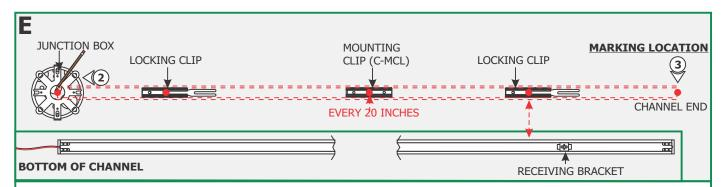
**NOTE:** Remote power supply must be installed within 40ft of Junction box. The low voltage 24V DC wires must be present in Junction box before installing the channel. Refer to the installation instructions provided with the power supply. See page 6 for wiring diagram.
