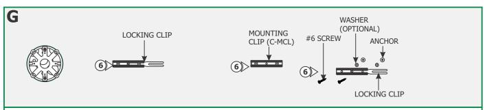
**6:** Line up the locking clips & mounting clips to anchor holes and secure them by tightening the two #6 screws through the clip holes followed by the washers into the anchors.
