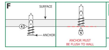
**NOTE:** Steps 3 and 4 are for drywall mounting. Omit these steps if mounting the clips to a wood surface directly.
