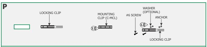
**12:** Line up the locking clips & mounting clips to anchor holes and secure them by tightening the two #6 screws through the clip holes followed by the washers into the anchors.
