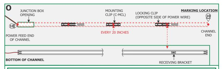
**NOTE:** If the receiving bracket interferes with the Junction box, then relocate the bracket by loosening the set screws and make the necessary adjustments.
