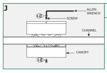
**12:** Place each canopy piece against the channel & line up the canopy hole with the crossbar hole. Secure the canopy in place with the screw & Allen wrench provided.
