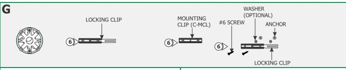
**6:** Line up the locking clips & mounting clips to anchor holes and secure them by tightening the two #6 screws through the clip holes followed by the washers into the anchors.
