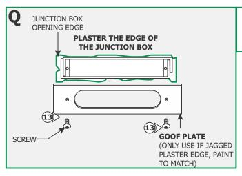
**13: Optional:** Use the Goof Plate if the junction box opening has a lot of imperfection/jagged edges. Install the provided goof plate (paint to match prior) with the two screws.
