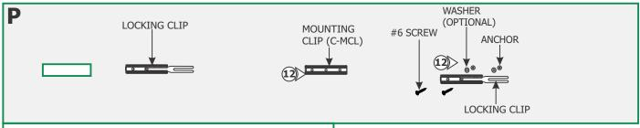
**12:** Line up the locking clips & mounting clips to anchor holes and secure them by tightening the two #6 screws through the clip holes followed by the washers into the anchors.
