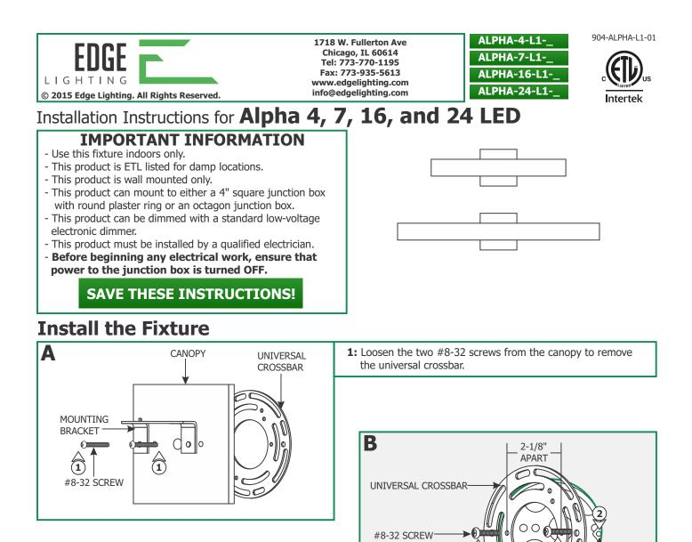
2: Mount the universal crossbar to the electrical box holes with the provided #8-32 screws so that the two inner threaded holes (spaced 2-1/8" apart) on crossbar are leveled horizontally.
