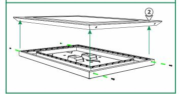
**3:** Align the mounting plate hole with the power line conduit, or junction box. Use the mounting plate as a template to mark eight mounting holes (highlighted in GREEN) onto the wall.
