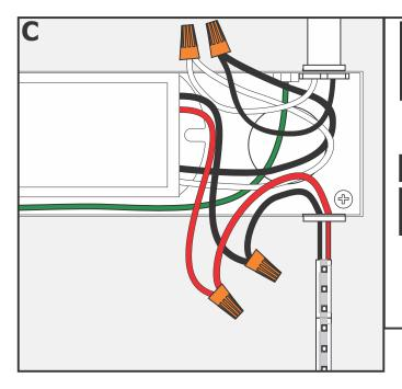
**NOTE:** In order to use small gauge wires from the power supply to the LED fixture, it is recommended to install the power supply as near as possible to the LED fixture. See "Low Voltage Wire Size Chart" below.
