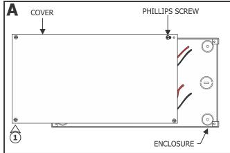
**1:** Loosen the four Phillips screws on the front of the power supply cover to slide the cover off of the enclosure.
