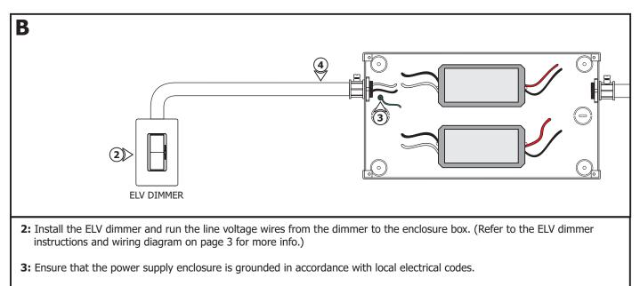
4: Remove knockouts from power supply enclosures as required. Route 120VAC hot and neutral wires from the ELV dimmer to power supply enclosure.
