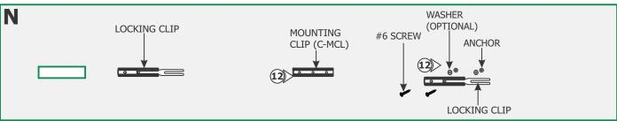
**12:** Line up the locking clips & mounting clips to anchor holes and secure them by tightening the two #6 screws through the clip holes followed by the washers into the anchors.
