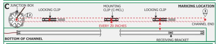
NOTE: Remote power supply must be installed within 40ft of Junction box. The low voltage 24V DC wires must be present in Junction box before installing the channel. Refer to the installation instructions provided with the power supply. See page 5 for wiring
