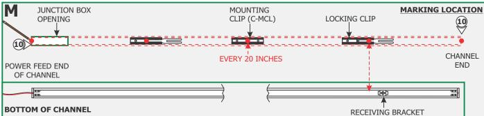
**NOTE:** If the receiving bracket interferes with the Junction box, then relocate the bracket by loosening the set screws and make the necessary adjustments.
