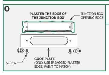
13: Optional: Use the Goof Plate if the junction box opening has a lot of imperfection/jagged edges. Install the provided goof plate (paint to match prior) with the two screws.
