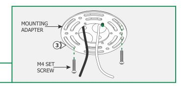
**3:** If required, secure the mounting adapter to the electrical box holes with the two #8-32 screws provided.
