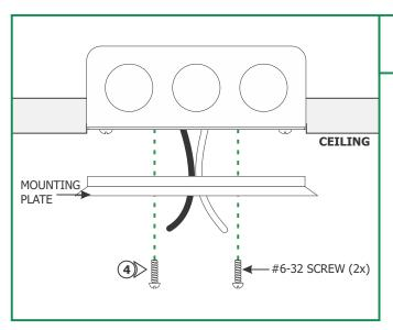
**4:** Feed the power wires through the center hole of the mounting plate and secure the plate to the mounting adapter using supplied 6-32 screws.
