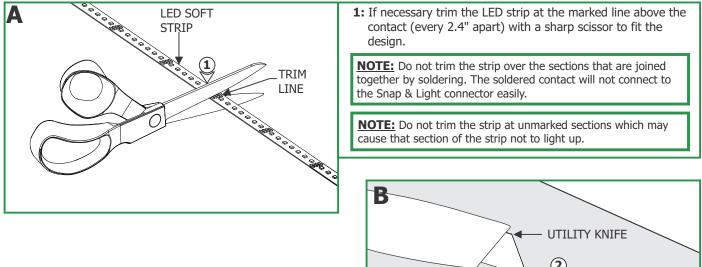
**2:** Place the LED Soft Strip on a flat, stable surface. Using a utility knife, carefully scrape the protective coating from the contacts.
