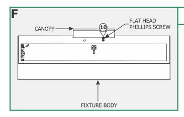
**10:** Secure the right fixture body hole with the flat head Phillips screw provided.
